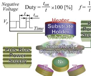
Fig.: Schematic illustration of RF magnetron sputtering system using separate elemental targets with a heating and ion-irradiating system for substrates. The ion irradiating system was actually utilized plasma-based ion implantation.
