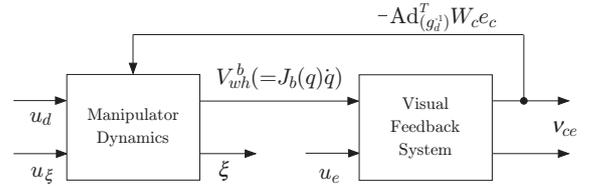
Figure 3: Block diagram of the dynamic visual feedback system
