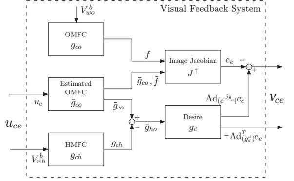
Figure 2: Block diagram of the visual feedback system
