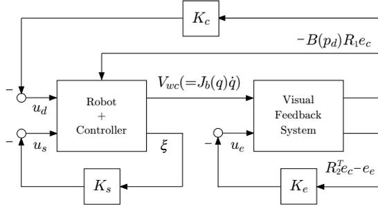
Figure 5: Block diagram of dynamic visual feedback control.
