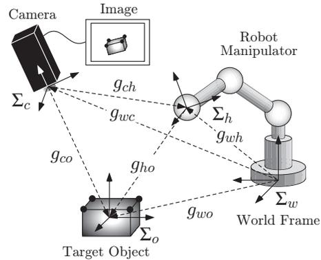
Fig. 1. Visual feedback system with a fixed camera.
