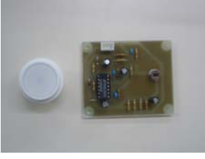
Fig. 2. Conventional pyroelectric infrared sensor and fresnel lens.
